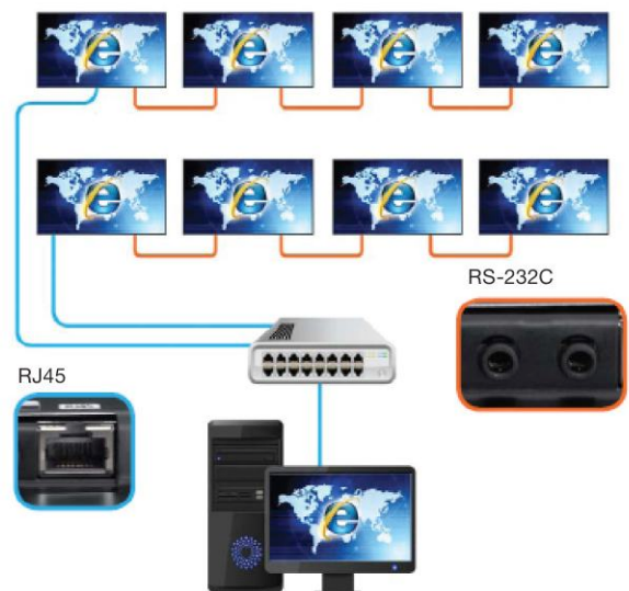
Figure 4. Samsung MD65C LED displays enable RJ45 and RS-232 connectivity simultaneously.
